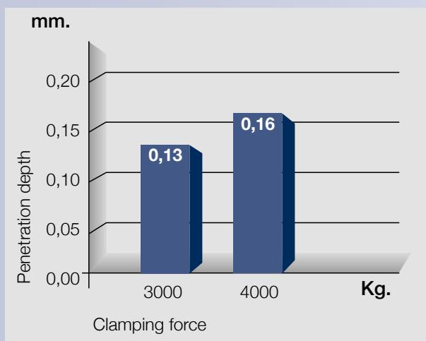
Steel with tensile strength  $\approx 980 \text{ N/mm}^2$
