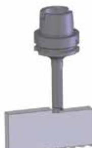
Mill the jaws to the necessary height
