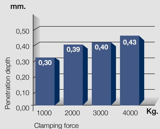
The same proportion is comparable to the clamping surface for only 2 mm, that is with one row of teeth per insert (see chart).
