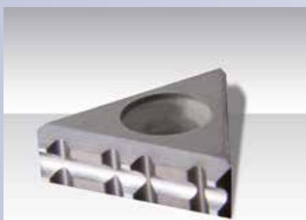
In a general sense, the insert with its own special section of pyramid shape and special teeth sharpening penetrates into the material of the workpiece and creates some coupling without any clearance, unloading the forces and the vibrations, becoming a sole body with the vise and the workpiece.
