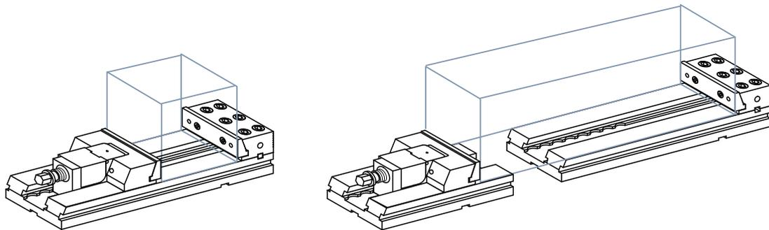
The modularity of the system combined with some other components offers many additional clamping solutions.
