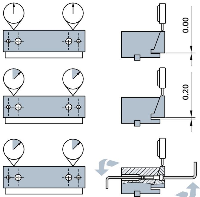
**How to clamp the vises at the table of the machine tool.**
